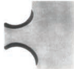
双排异径球式鼻圈滚道 Double-row different diameter ball type nose ring raceway
