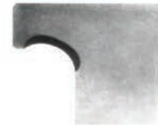
双排异径球式压圈滚道 Double-row different diameter ball type pressure ring raceway
